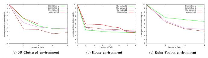
Fig. 3: We show a decrease in the average hausdorff distance between paths as the number of coarsely diverse paths increase. For our method U = Uniform topological planner, G = Gaussian topological planner, and B = Bridge-Test topological planner.
